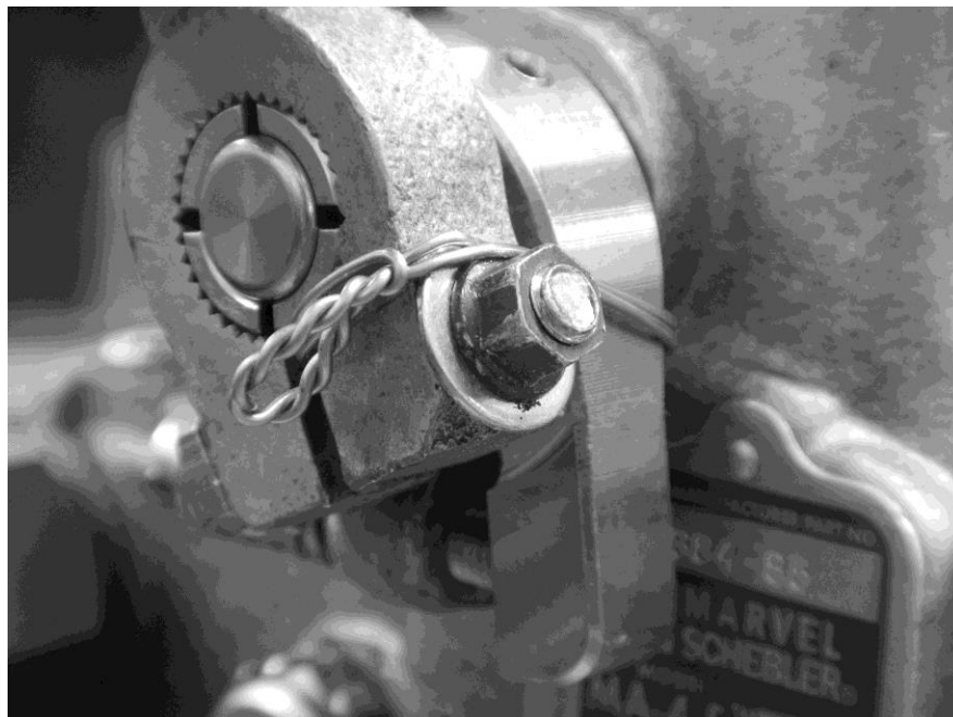
Figure 5-11d: Safety Wiring of Throttle Arm to Carburetor Stop Arm
